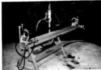
Jack leg being tested by itself. Special air inlet adaptors allow operators to inject or release air.
