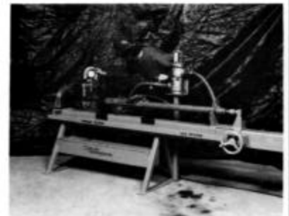
Drill Doctor checking jack leg operation.
